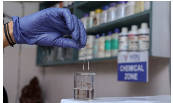
Chemical Analysis for Fibre Identification
