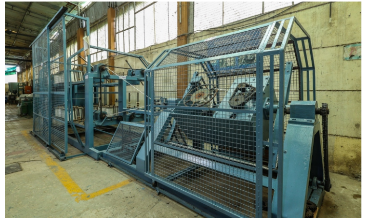
Twisted Rope making ( 3 & 4 Strands ) 8 - 20 mm Dia
