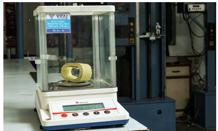
Electronic Weighing Balance (0.001g & 0-220g)
