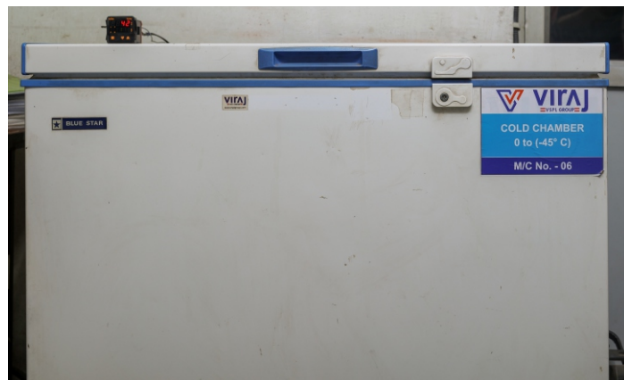
Cold Conditioning Chamber upto - 45 degree
