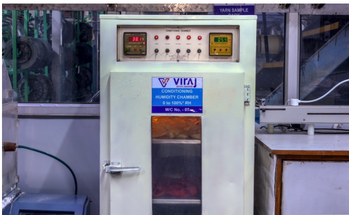
Conditioning Chamber with thermostat Range (0-110° C)
