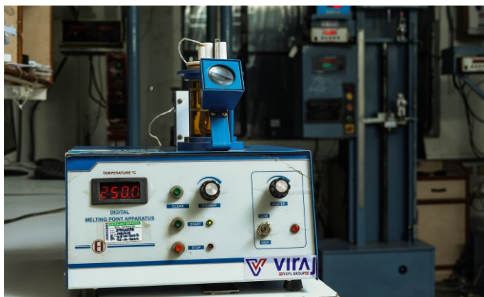
Digital Yarn Melting Point Testing
