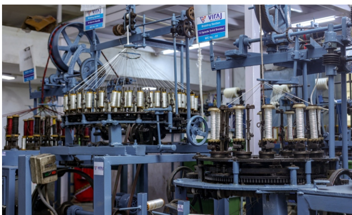
Solid 12 spindle Braiding M/c
