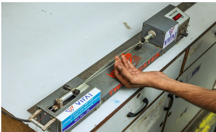
Twist Tester Motorized (0-99999 counts)
