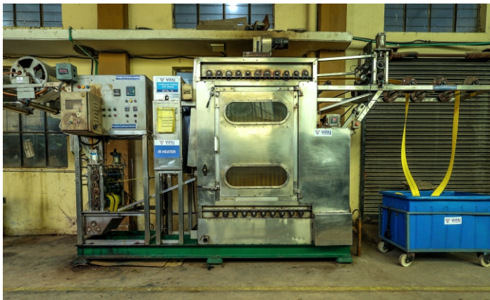
Continuous Dyeing M/c for Nylon (Steaming Process)
