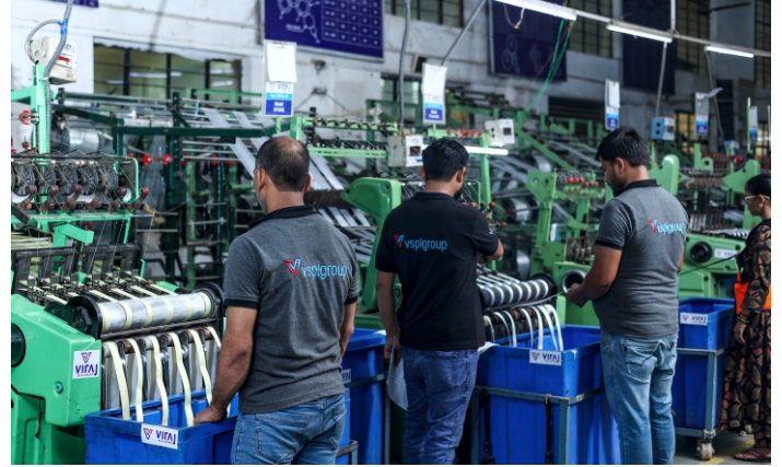
Automatic High speed Needle Looms (Shuttle-Less Loom)
