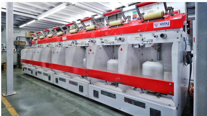
Computerised high speed precision Yarn twisting M/c
