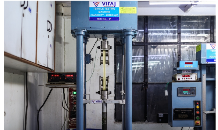
Digital Tensile Testing Machines (20,000 Kgf max)
