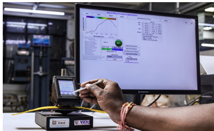
Spectrophotometer for shade matching testing
