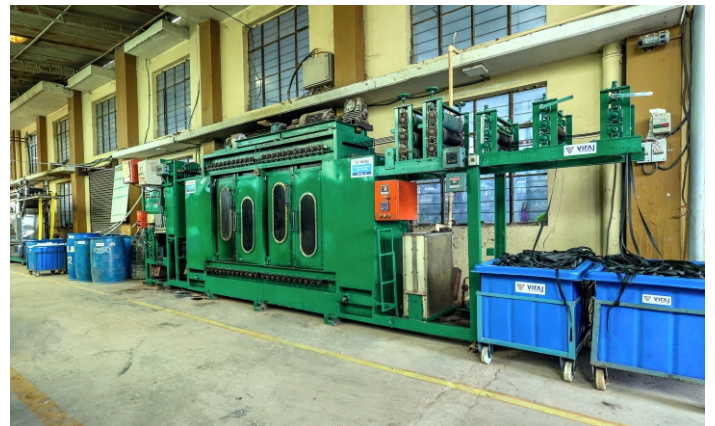
Continuous Dyeing M/c for Polyester (High Temp hot air circulated Process)
