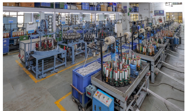
High Speed 12, 16, 32 & 48 spindles Braiding M/c
