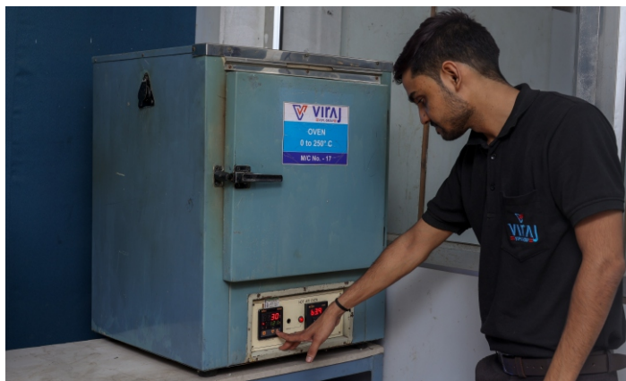
Oven with timer and Temp. Control (1° C - 250° C)
