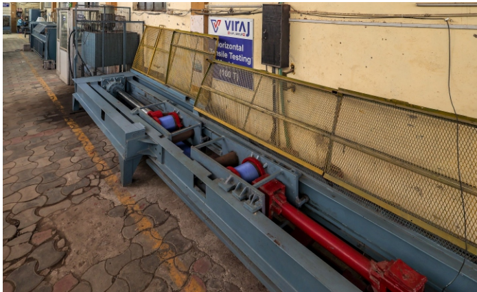
Digital Tensile Testing Machines (100,000 Kgf max)
